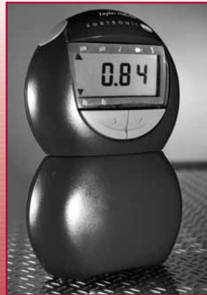
Figure 2 Surface Micro- roughness Meter
