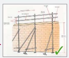
**Fragile roofs:** always follow a safe system of work using a platform beneath the roof where possible. Work on the roof requires a combination of stagings, guard rails, fall restraint, fall arrest and safety nets slung beneath and close to the roof.
