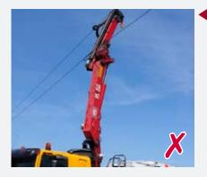
The jib on this lorry has hit the overhead power line. Tipper lorries, lighting towers, excavators, scaffold tubes and metal ladders have all been involved in fatalities when contacting or coming into close proximity with overhead cables.
