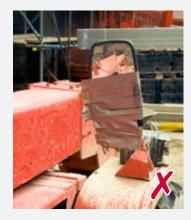
The wing mirror on this telescopic fork lift truck is damaged and obscured by tape. Incidents usually occur when plant is reversing or slewing so driver visibility is vital. Maintenance systems must be in place for checking brakes, steering, lights etc.
