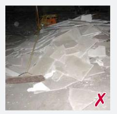
▲ This shows what can happen when a survey is not undertaken or the findings not acted upon. Asbestos insulation board is shown strewn on the floor having been swept with a broom.
