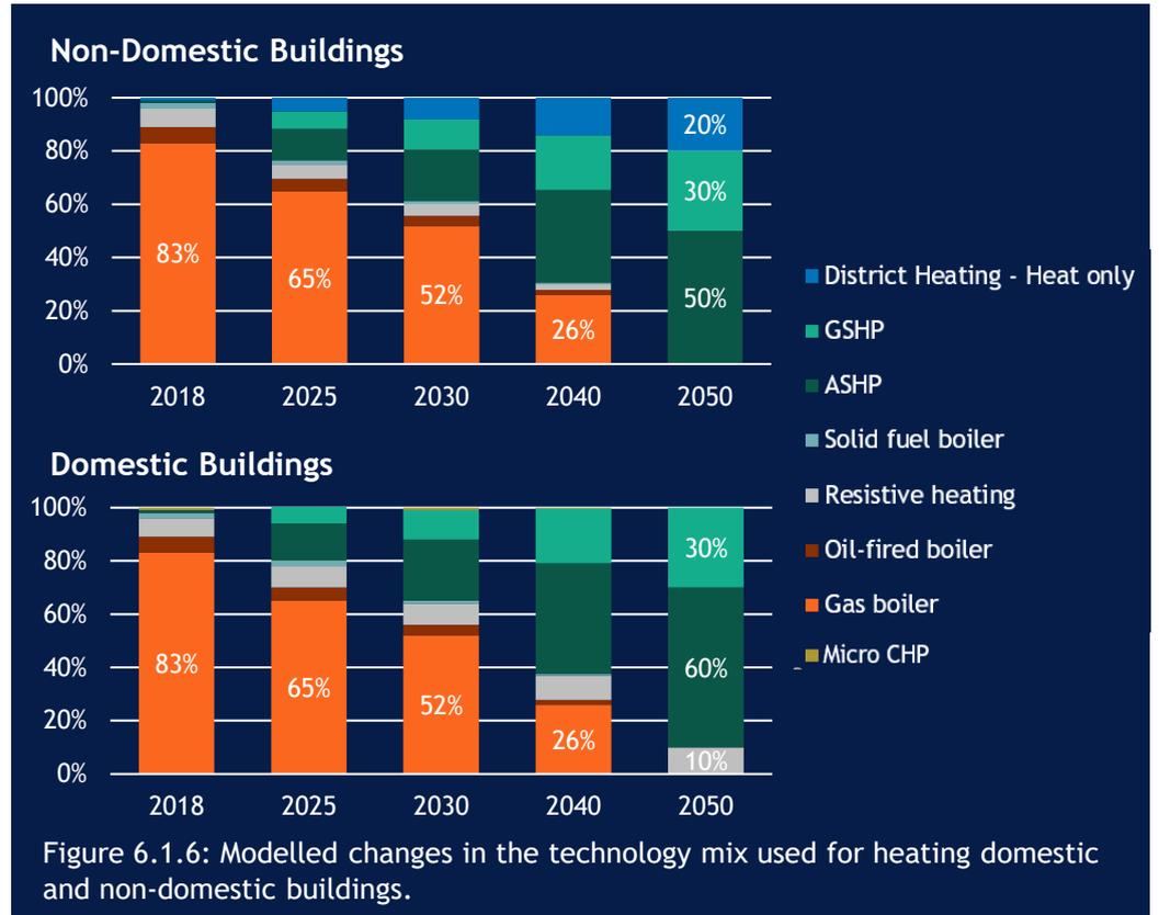
Figure 6.1.6: Modelled changes in the technology mix used for heating domestic and non-domestic buildings.
