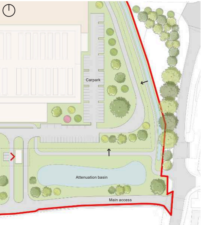
These plans are design explorations of the landscape configuration for the eastern side of the plot, near the main entrance, including layout changes for the car park, fence and attenuation basin. The fence location is indicated with a black arrow.
