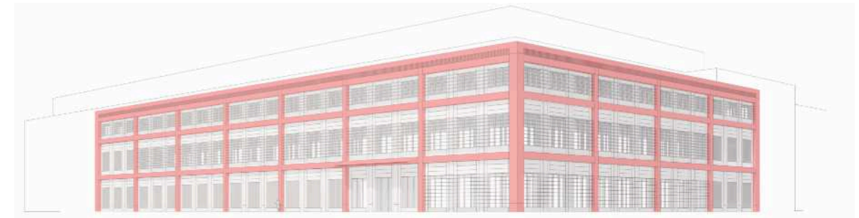
First Façade Hierarchy: Dark, beige-toned pre-cast deep elements define a 15 x 7 m structural frame on the ground and first floors, (15 x 4.3 m at second floor) establishing a prominent architectural rhythm.
